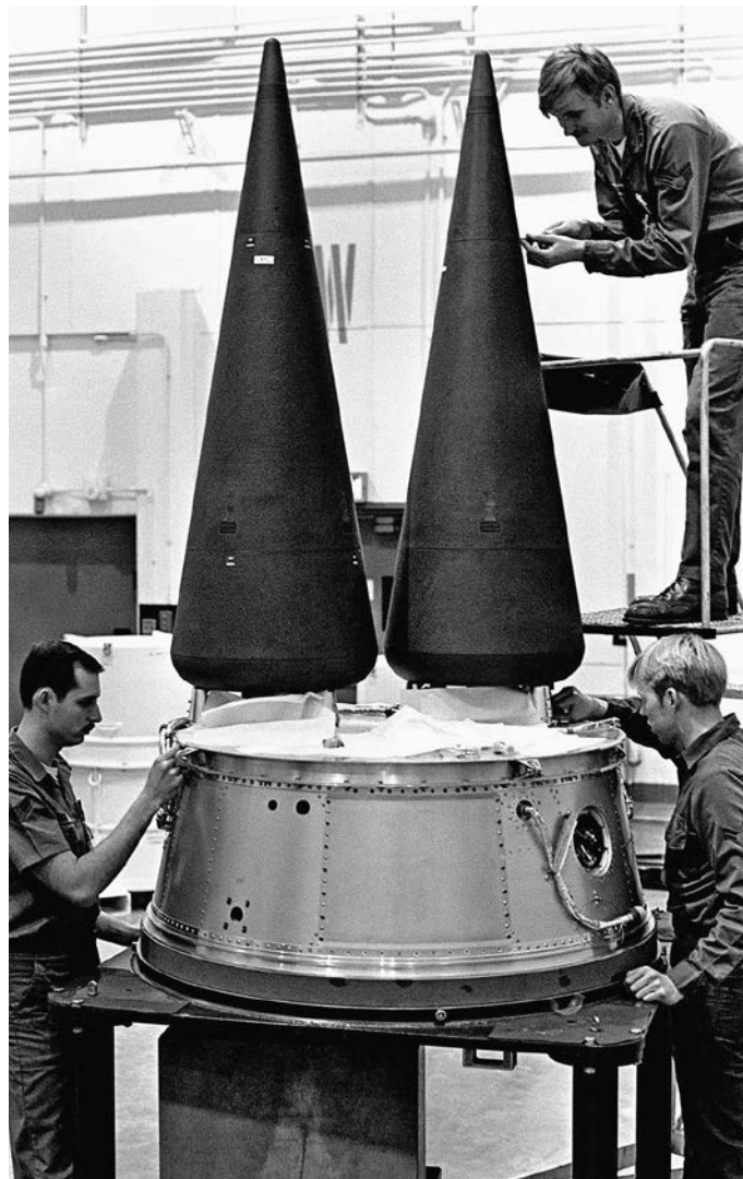
Airmen perform maintenance on the warheads and reentry vehicle of a Minuteman missile in the 1970s. National Museum of the US Air Force
